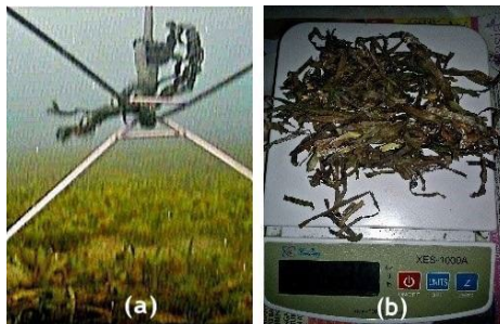
Figure 1: (a) A snapshot of seagrass sampling video using underwater camera; and (b) Dried-biomass measurement of seagrass sample.
