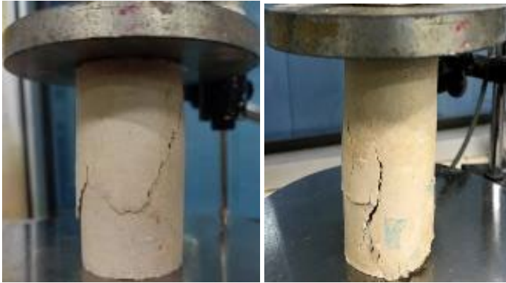
Figure 8: Comparison of shear failure for the untreated soil sample and the treated soil sample added with 1% of 10 x 30 mm of OLFM strips
