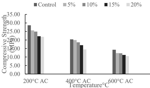
**Figure 6:** Compressive strength after elevated temperature exposure subjected to air cooling.
