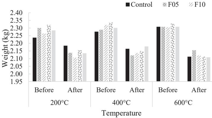
**Figure 4:** Mass loss of CBA concrete subjected to air cooling at 28 days of curing.
