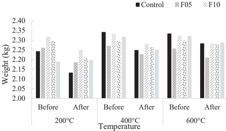
**Figure 5:** Mass loss of CBA concrete subjected to water cooling at 28 days of curing.
