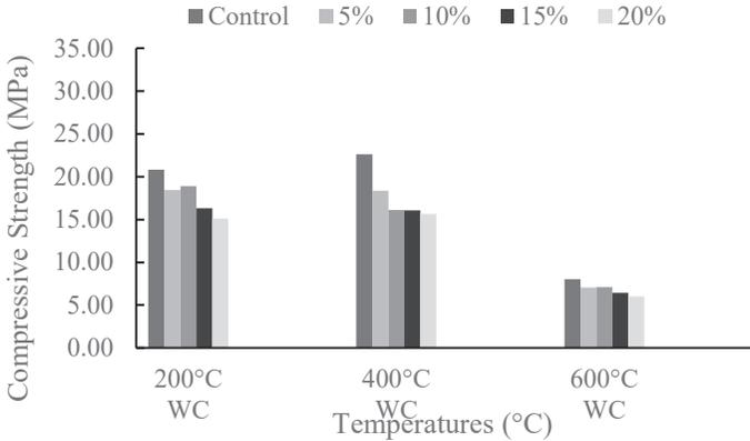
**Figure 7:** Compressive strength after elevated temperature exposure subjected to water cooling.
