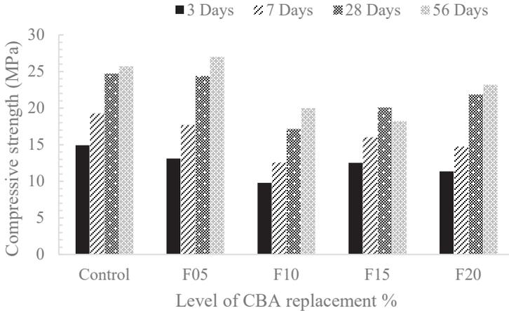
**Figure 1:** Compressive strength of pre-treated CBA concrete
