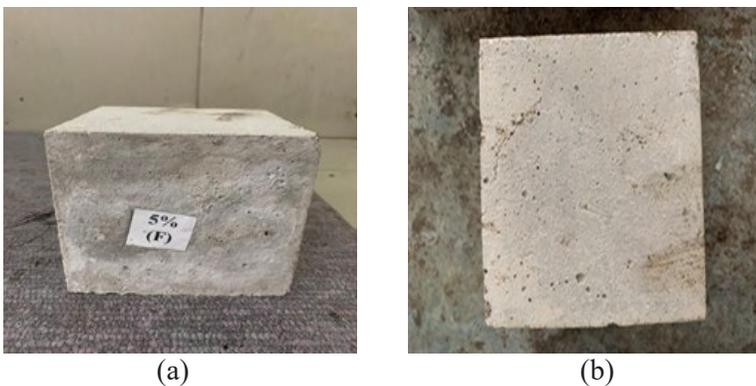
**Figure 2:** Appearances of F5% of CBA samples exposed to the air cooling at (a) 200 °C and (b) 400 °C temperatures.
