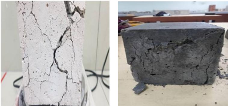
**Figure 3:** Appearances of F5% of CBA samples exposed to the air cooling at 600C temperature.
