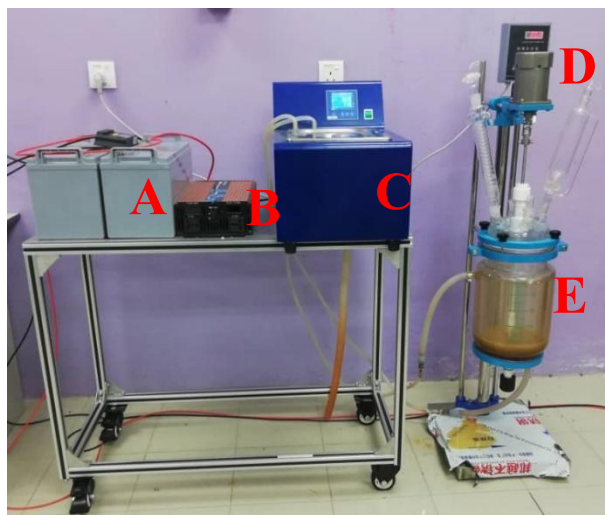
Figure 1: Experimental set-up for the Anaerobic Bioreactor (A: Battery, B: DC-AC Converter, C: Water Vapourisation, D: Stirrer Motor, E: Main Reactor).
